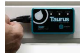
Step 1.4: Connect Cat 5e cable to remote
