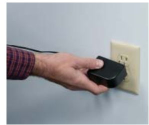
Step 3.1: Plug wall transformer into AC outlet
